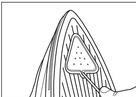
2. Using a Philips-head screwdriver, remove the three screws in the Heat Filter
