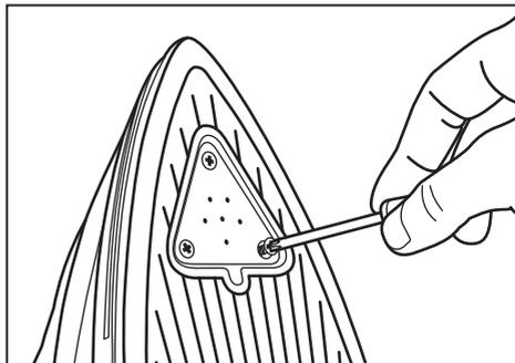
3. Remove the Heat Filter and clean with a brush to remove any blockages or debris inside.
